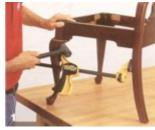
1) Break the joints apart. In many situations, you can disassemble a dowel joint with nothing more than a bar spreader and a non-marring mallet.
