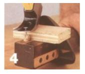
**4) Add a screw.** A dowel that's broken near the surface is tough to grip with pliers. So drive a small screw into the dowel, then pull it with a claw hammer.
