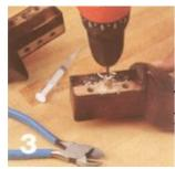
**3) Drill a hole.** If alcohol around the outside of the dowels has no effect, drill a hole into each one, and squirt alcohol inside. Wait a few minutes while it soaks through the wood, then try to yank out the dowel with pliers or side cutters.
