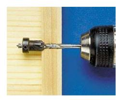
First reverse the countersink cutter on the end of the drill bit, as shown in the photo. Then insert the bit through the pilot hole and chuck it in the drill. Now to countersink the hole, all you have to do is reverse the direction of the drill and gently pull back on the bit.
