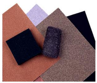
Basic abrasives are (clockwise from top left) garnet paper, aluminum oxide paper, silicon carbide paper, wet/dry paper, steel wool and abrasive pads.
